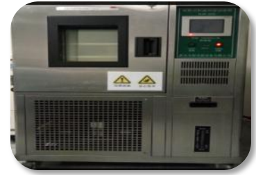
Programmable temperature and humidity chamber Function: Reliability test
