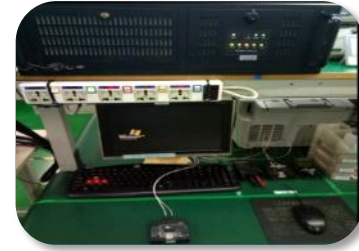
Pi-network crystal test system Function: Frequency, DLD and resistance test
