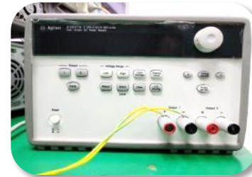
Stabilized voltage supplier Function : Provide DC voltage
