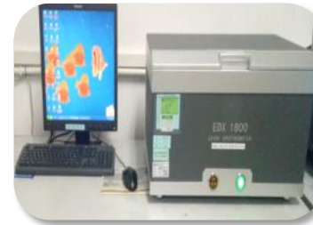
XRF Spectrometer Function: ROHS material test
