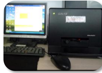
Crystal blank shape tester Function: Blank dimension measuring
