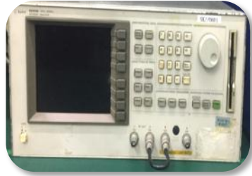
Network analyzer Function: Frequency and resistance test
