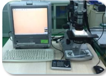
3D electronics microscope Function: Magnification rate :1200 times, Accuracy: 0.005mm
